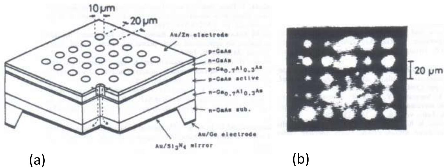
Fig. 8 Two-dimensional VCSEL array[A11]
