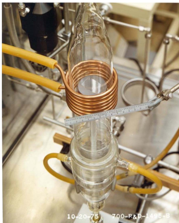
Fig. 2. Photograph of the MOCVD reactor chamber with a large-area (0001) sapphire substrate loaded on the 2.0-in diameter SiC-coated graphite susceptor. (Photograph taken on October 20, 1975.)
