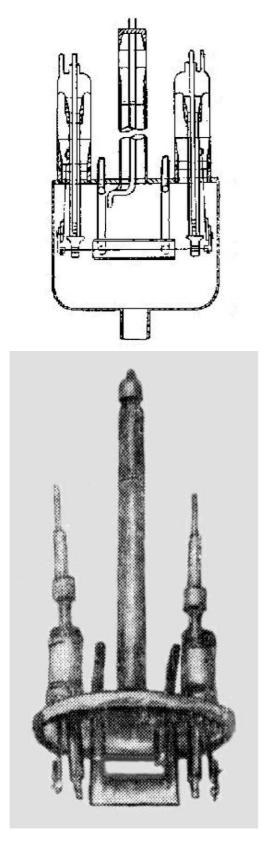
Figure 4. Water-cooled magnetron in metal case, circa 1934.
