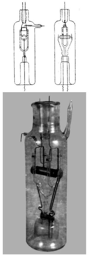
Figure 5. Non-cooled 60-kW magnetrom for 60 cm wavelength, 1935.
