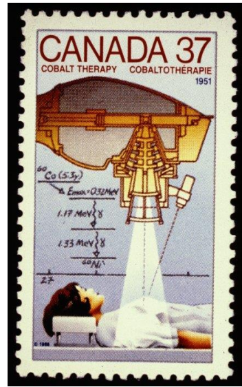
Figure 14. Canadian postage stamp recognizing the development of cobalt-60 radiation therapy in Canada and the involvement of Harold Johns in that development. The stamp includes a schematic of a typical head of a cobalt-60 machine. The source shutter mechanism is a sliding drawer. The source is shown in the “on” position. To turn the beam “off”, the source drawer is slid to the left. Also shown is the decay scheme of cobalt-60 with a beta decay with a maximum energy of 0.32 MeV followed by 2 gamma rays of 1.17 and 1.33 MeV. This style of machine was the most produced and used globally. Canada Post © 1988. Reproduced with permission.
