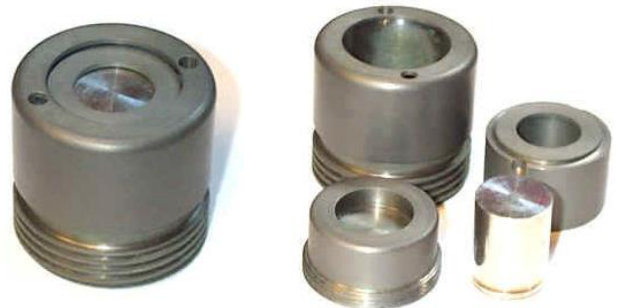
Figure 12. Cobalt-60 source capsule. The assembled source is shown on the left. The source components are shown on the right. The cobalt source itself is shown on the lower right-hand corner of the right figure and is about 2.5 cm in diameter whereas the total capsule is about 5 cm in diameter. The top of the source housing (on the left) contained an opening through which the stainless-steel source container can be seen. From [100].
