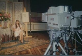
HDTV camera composed of 1-inch DIS (Diode-gun Impregnated-cathode SATICON) tube, at a CBS studio, 1982.
