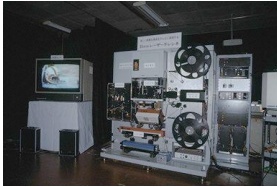
35-mm film laser telecine for converting film to HDTV, 1984.
