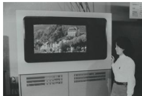
Wide screen display composed of three 26-inch CRTs, 1975.
