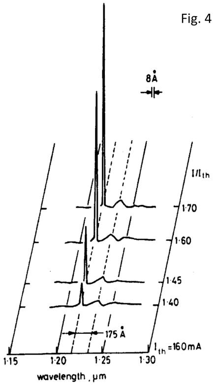
Fig. 4 Emission spectra of surface-emitting laser with a short cavity length[A8]
