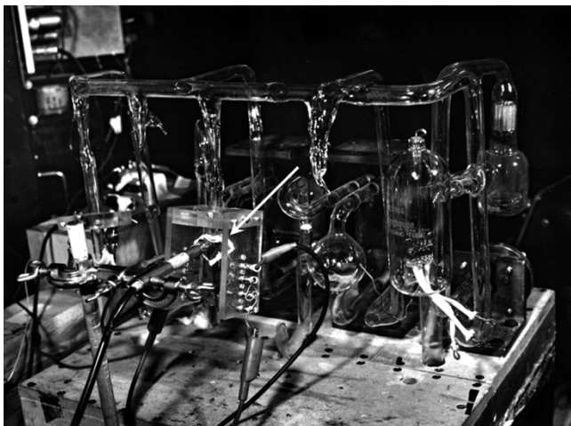
Fig. 2. Early plasma panel attached to the glass vacuum system used for the first plasma displays at the University of Illinois. Arrow points to the 1-in \times 1-in panel. This had the same alternating sustain voltage, neon gas, and dielectric glass insulated electrodes that we use for plasma TVs today. Wall charge that collected on the dielectric walls allowed it to have inherent memory—just as today. Photo from [12].
