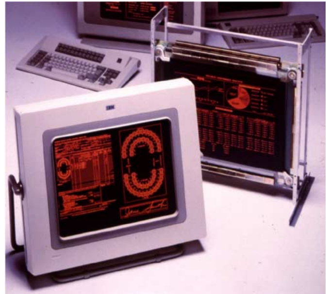
Fig. 16. Monochrome 960 \times 768 pixel plasma display product line introduced by IBM in 1983 [28]. This 17-in diagonal display could present the information of four normal computer displays of that era.
