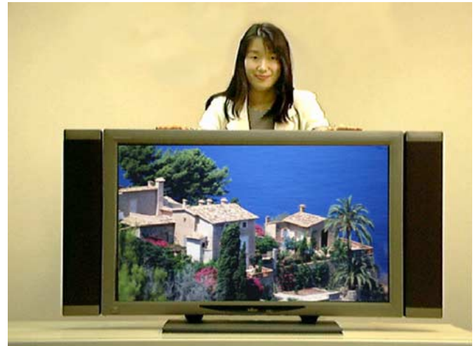
Fig. 25. First 42-in full color product introduced by Fujitsu in 1995 [40]. All of today's plasma TVs followed the lead of this product and 42 in is still the most popular size today.
