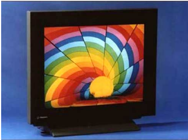
Fig. 24. The 21-in diagonal prototype developed by Plasmaco in 1994, having very high dark room contrast ratio. This uses a ramp waveform to generate a Townsend discharge mode [38], [39]. This accomplished the critical priming job without significant background glow.
