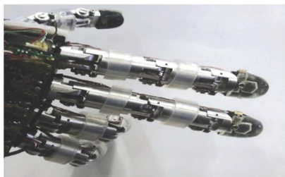
Fig. 5 Sensors installed in the fingertips of the iCub [17]
