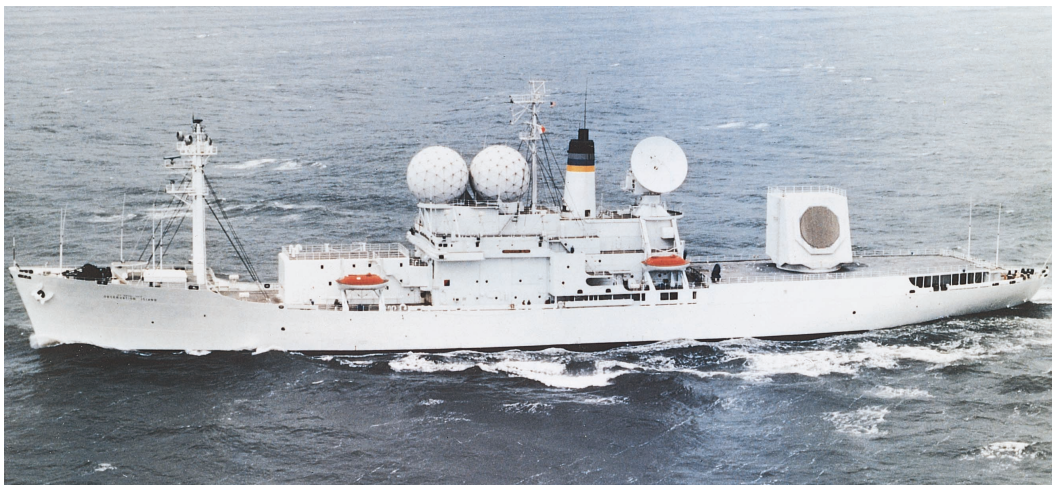
FIGURE 7. The wideband phased-array Cobra Judy radar on the U.S. Naval ship Observation Island . The S-band phased-array radar is at the stern of the ship; the mechanically scanned dish just forward of it is the X-band radar antenna. The Cobra Judy is the world's largest mobile phased-array sensor.
