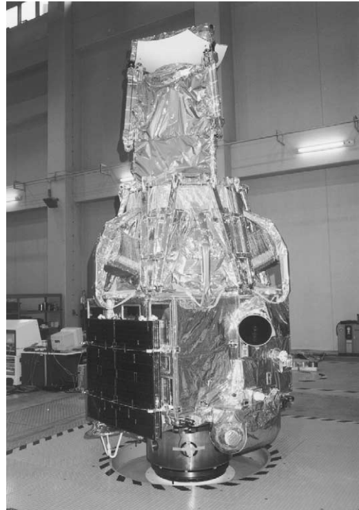
Fig. 2. HALCA before launch. The height is about 4 m and the total (wet) mass is 830 kg.
