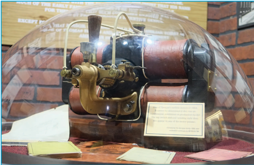
figure 1. The restored 1884 Sprague dc motor in the museum display. (Photo courtesy of Jeff Hakner, Shore Line Trolley Museum, operated by the Branford Electric Railway Association, East Haven, Connecticut.)
