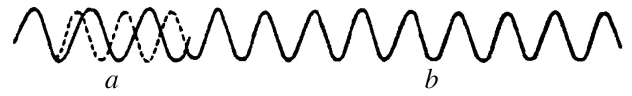
Fig. 6. Measured waveforms of the time dependence of (a) ac current of the Straßburg power station, (b) tuning fork oscillation [2].
