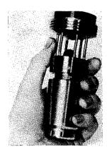
hydrostatic impulse forces mercury through a capillary passage and into a collector; the weight of mercury discharged is proportional to the impulse per unit area in p.s.i.-sec., from 10 to 400 p.s.i. The gauge is entirely self-contained and of simple construction, for convenience in field use. Its applications include geophysics, internal combustion studies, blast damage determination, and water hammer research.-Engi-NEERING RESEARCH ASSOCIATES, Inc., St Paul 4, Minnesota.
