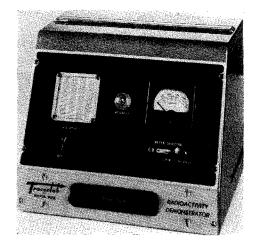
A removable shield is mounted in front of the Geiger tube, to completely eliminate beta-rays when it is desired to measure only gamma-radiation. A switch permits the meter also to indicate the voltage across the Geiger tube which can be varied from about 500 to 1100 volts. The instrument operates on 110 volts a.c.
