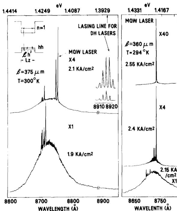
FIG. 2. (a) Lasing spectra for a MQW laser  $375 \mu\text{m}$  long and  $200 \mu\text{m}$  wide at two current injection levels. The inset shows the typical lasing spectra near threshold of a MBE grown conventional DH laser ( $375 \mu\text{m}$  long,  $200 \mu\text{m}$  wide, and  $0.4 \mu\text{m}$  active layer thickness) operated under similar conditions (b) Single-longitudinal operation of a broad-area MQW laser.
