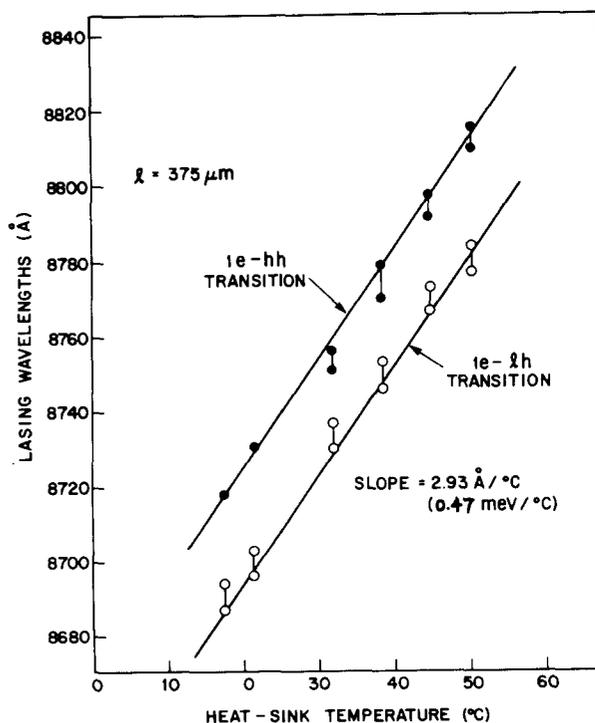
FIG. 3. Lasing spectral behavior of the 1 e-lh and 1 e-hh transitions for the same MQW laser given in Fig. 2(b) as a function of heat-sink temperature near the lasing threshold for the 1 e-hh transition. The solid and empty dots indicate the wavelengths of the dominant longitudinal modes for each confined-particle transition.
