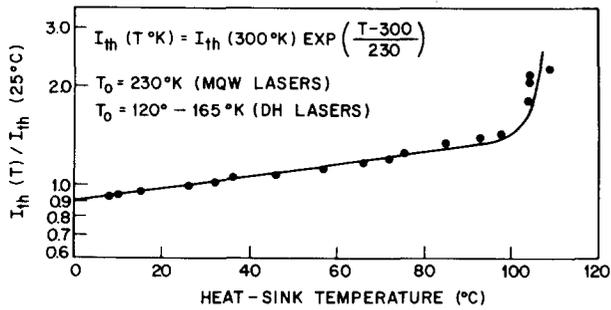
FIG. 4. The pulsed current threshold for the 1 e-hh transition as a function of heat-sink temperature for a typical MQW laser.
