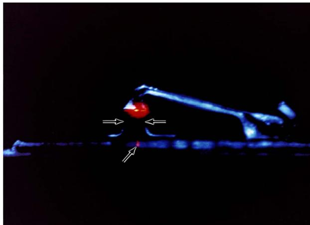
**Fig. 4. First (1962) red-spectrum GaAsP diode laser with its red output photographed directly on film without electrical detector conversion. The yellow spot is the overexposed output-beam center, with the true red coherent signal output shown off-angle at reduced intensity by the lower reflected diffraction spot.**
