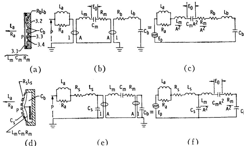
Fig. 3. Pressure microphone with displacement-responsive transducer.
