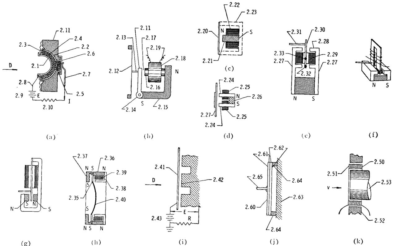
Fig. 2. Various types of transducers used in microphones.
