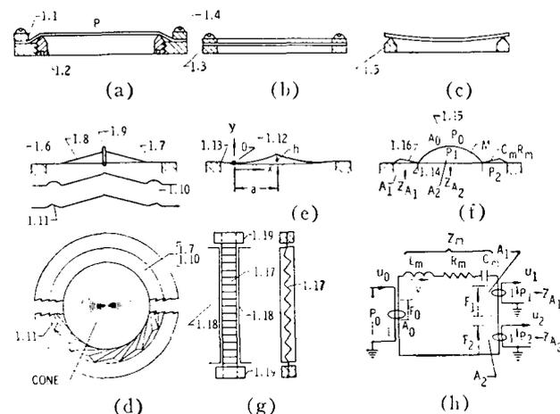
Fig. 1. Various types of diaphragms used in microphones.
