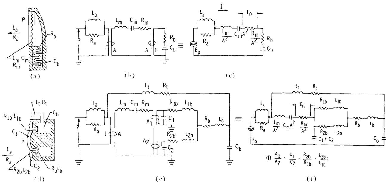
Fig. 4. Pressure microphone with velocity-responsive transducer.
