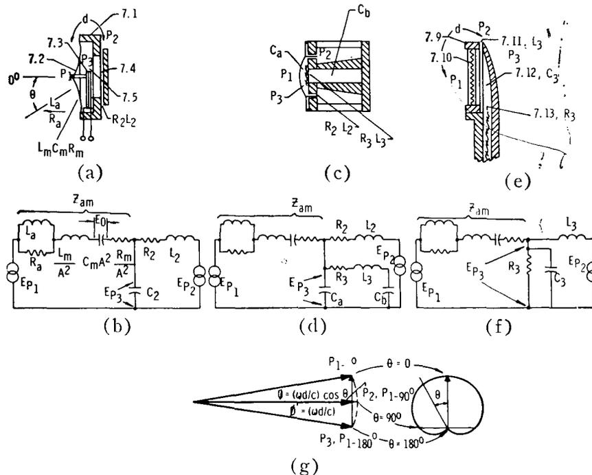
Fig. 7. Phase-shift unidirectional microphones.
