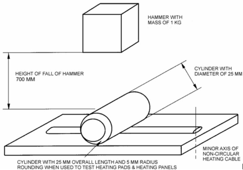
Figure 2—Trace heater room temperature impact test apparatus
