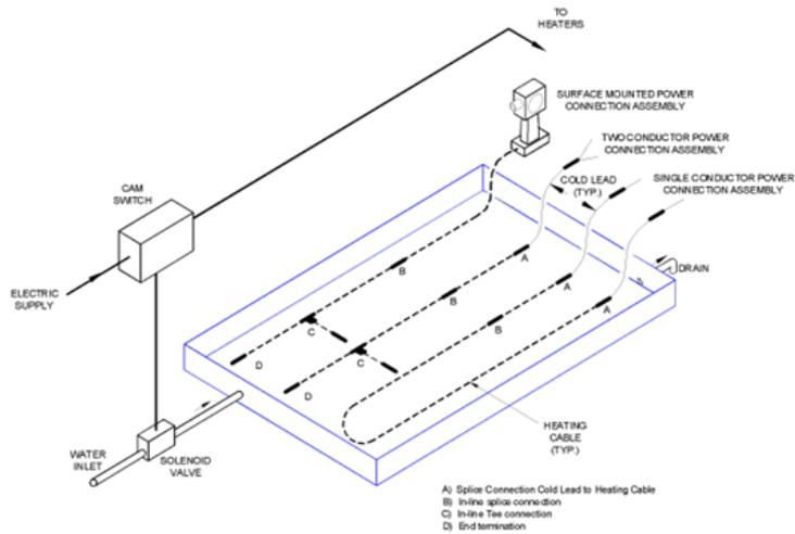
Figure 1—Trace heater termination and splice test apparatus
