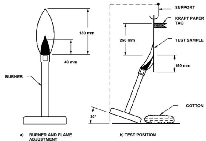
Figure 4—Flammability test
