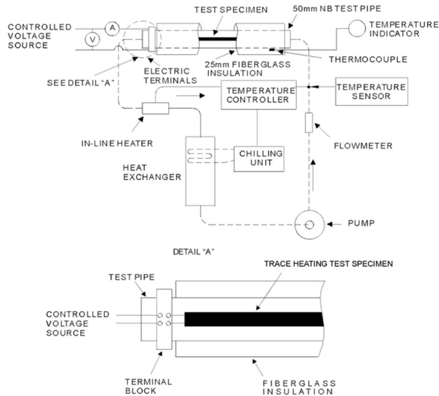
Figure 5—Verification of rated output
