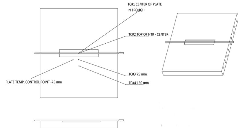
Figure 7—Verification of sheath temperature, plate test
