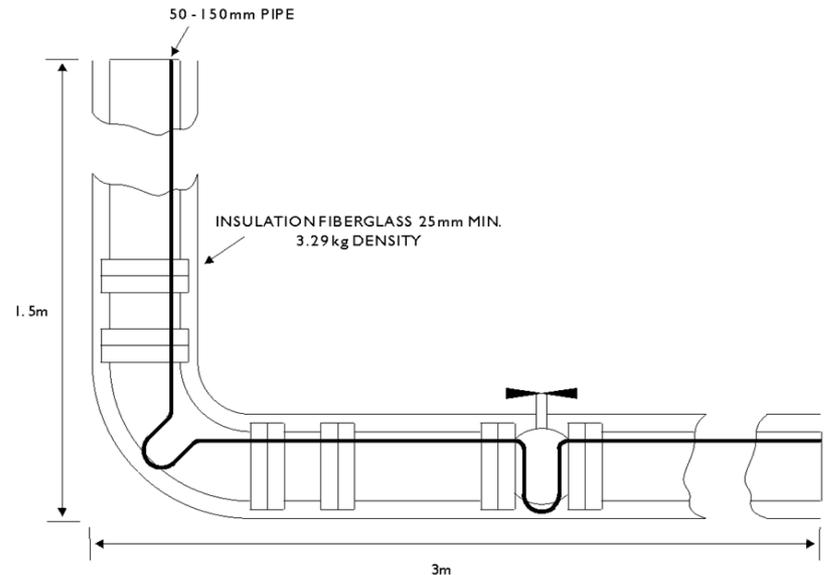
Figure 6—Verification of sheath temperature using systems approach
