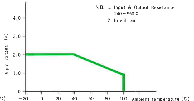
Range of suitable input voltage on constant voltage drive
