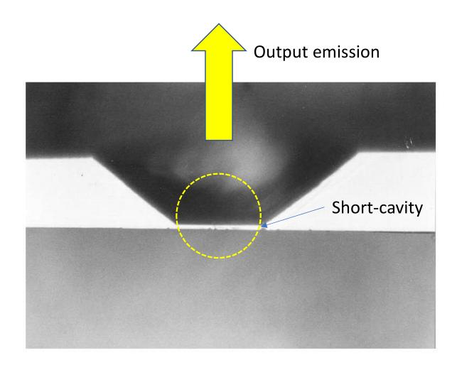
Fig. 3 A cross section image of a short cavity VCSEL. Thickness of the center etched portion is about 10 microns.
