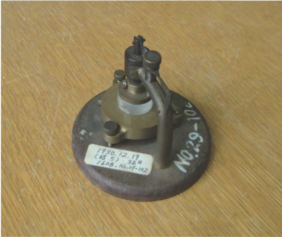
Fig. 3 Crystal plate holder apparatus used by Koga in his early research (1930)
