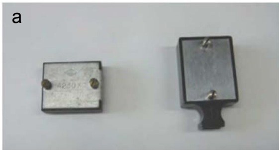
Plug-in types widely used in conventional transmitters
