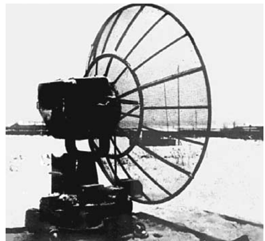
Figure 1. Single-antenna L -band pulsed radar "Zenit," developed in UIPT (1938-1943).
