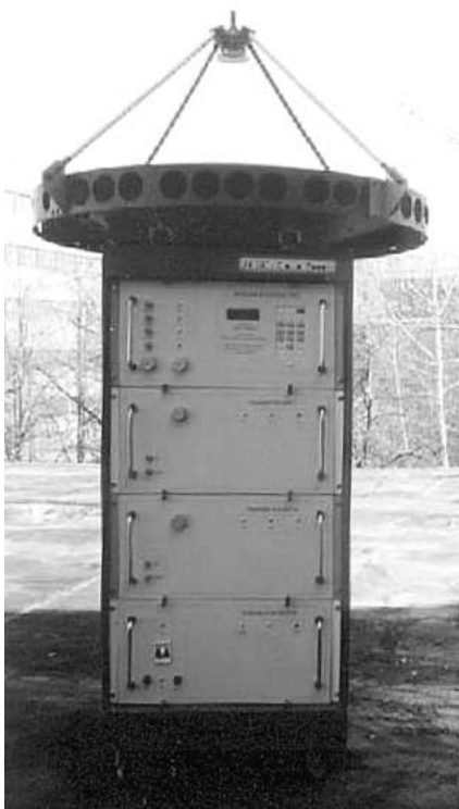
Figure 3. Outdoors photo of the 36-GHz cloud radar developed in IRA NASU in collaboration with METEK, Germany (2000).
