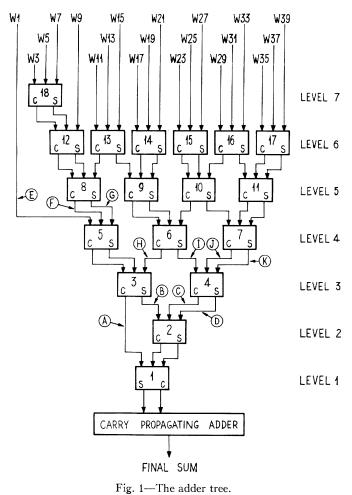
$(W_1 \text{ to } W_{39})$  and express their sum as the sum of two numbers. These are shown added in a conventional carry-propagating adder to produce the final product. The design of this adder will not be discussed, as several excellent designs having carry-propagation times of the order of 100 nsec have been devised [1], [5].
