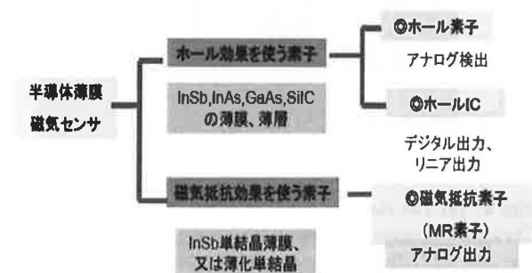
Fig. 2 Family of the semiconductor magnetic sensors.
