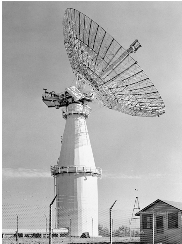
FIGURE 5. An early photograph of the antenna and supporting pedestal of the long-range UHF missile- and satellite-tracking radar on Millstone Hill in Westford, Massachusetts.
