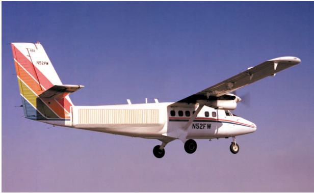
FIGURE 14. Flight test of the Multiple-Antenna Surveillance Radar on a Twin Otter aircraft. The rectangular displaced-phase-center antenna can be seen on the fuselage behind the wing.
