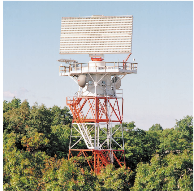
FIGURE 19. The ultralow-sidelobe UHF radar antenna under test on Katahdin Hill, Lexington, Massachusetts. This antenna is 5 \times 10 m in size.
