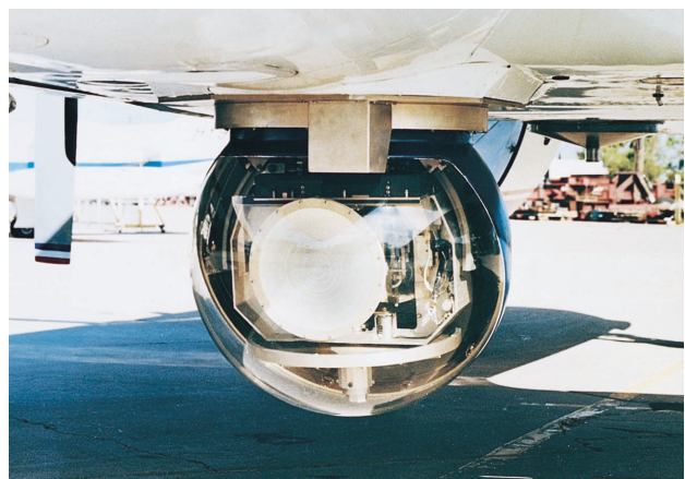
FIGURE 15. The Advanced Detection Technology Sensor (ADTS) airborne radar, a fully polarimetric, high-resolution synthetic-aperture radar (SAR) mounted below the fuselage of a Grumman Gulfstream aircraft.
