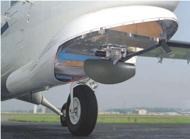
FIGURE 16. The unmanned-air-vehicle (UAV) moving-target-indicator radar system mounted in an Amber UAV fuselage attached to a Twin Otter aircraft. The radome has been removed from the UAV to show the radar antenna.
