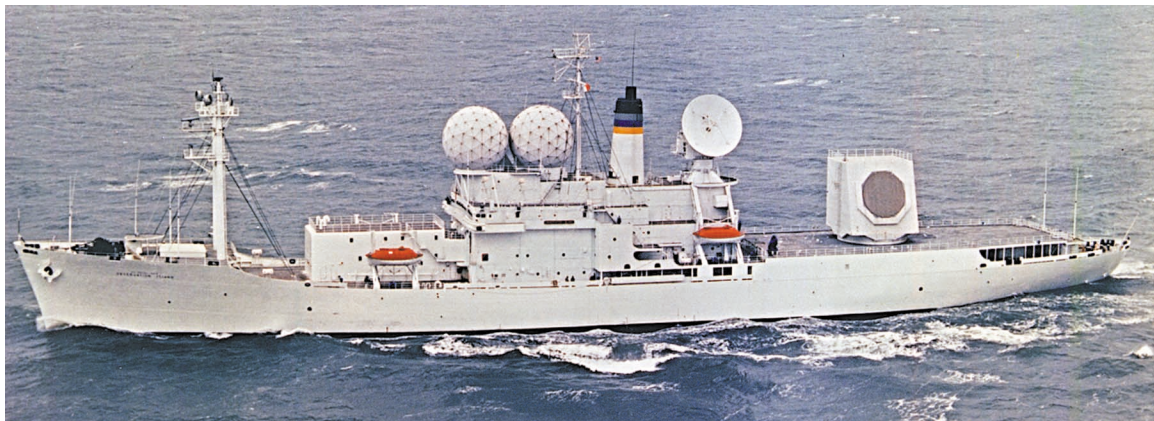
FIGURE 10. The Cobra Judy phased-array radar (far right) in its sea-based configuration on the USNS Observation Island . Putting a radar such as Cobra Judy on a mobile platform adds greatly to a radar's flexibility and utility.
