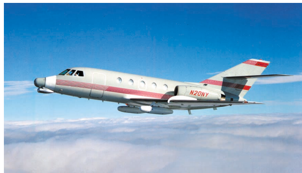
FIGURE 18. The Airborne Seeker Test Bed, or ASTB, installed in the nose and under the fuselage of a Gulfstream jet aircraft. The ASTB allowed researchers to emulate a surface-to-air missile or an air-to-air missile, thus making the ASTB essentially a flying missile-seeker laboratory.
