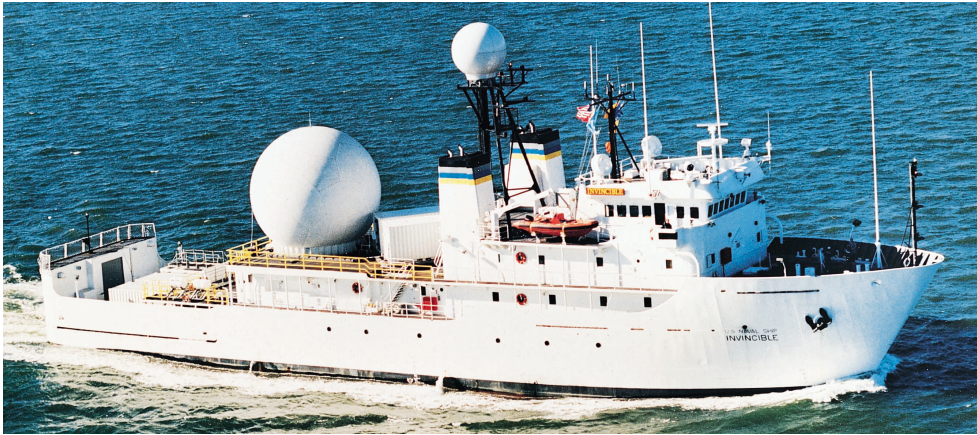
FIGURE 11. The Cobra Gemini radar antenna (inside the large radome) in its sea-based configuration on a T-AGOS-class ship, the USNS Invincible . The flexibility of a mobile platform allows Cobra Gemini, like Cobra Judy, to be deployed where it is needed and when it is needed.
