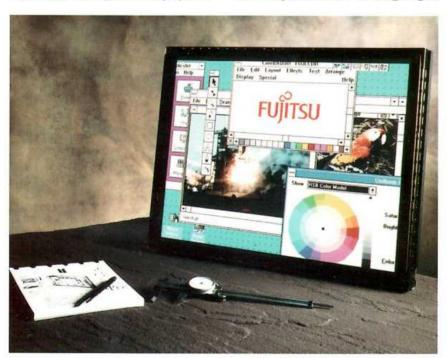
Joining in the race to oust the CRT in high-information-content display applications, the FPF21C806UA-02 is the first large-screen plasma display to reach the commercial market.
