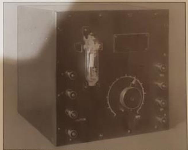
Fig. 28. Early prototype detector using a Marconi V24 valve
