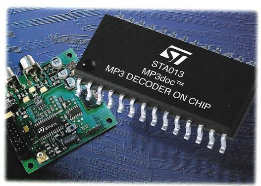
Portable MP3 audio players like Saehan's "MP3Man" and Diamond Multimedia's "Rio" store compressed audio files in flash memory and play it back through an MP3 decoder chip. No mechanism, tape or disc is needed. ST's new STA013 MP3 Audio Decoder IC is aimed at players like this and offers the lowest consumption on the market.
