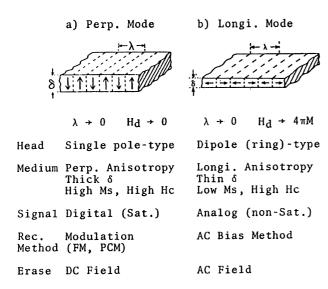
Fig. 15. Complementary relation between perpendicular type recording and longitudinal recording.  $^{10)}$
