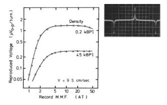
Fig. 14. Saturation characteristics for a double-layered medium showing no reproduced amplitude reduction at high densities (45 kBPI), even for excess recording magneto-motive forces (M.M.F.). The waveform is for a 200 BPI signal, being the same mono-pulse as that in longitudinal recording.
