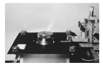
Fig. 10. Perpendicular flexible disk drive with a Co-Cr/Ni-Fe double layered recording medium and a single pole head. The auxiliary magnetic pole was located on the rear side of the disk.
