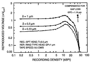
Fig. 11. Reproduced voltage versus linear bit density characteristics for perpendicular magnetic recording with various recording layer thickness,  $\delta$ .
