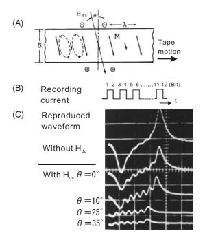
Fig. 4. Magnetization mode transformation by application of a dc magnetic field. (A) Method of mode transformation, (B) Recorded current, (C) Playback waveform variation by application of the dc field (M, magnetization for recording;  $H_{\rm dc}$ , applied direct current magnetic field; and  $\theta$ , angle of  $H_{\rm dc}$  from the recording medium plane).
