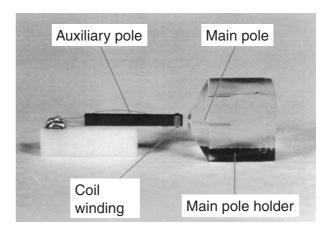
Fig. 7. Auxiliary-pole driven single-pole type head.
