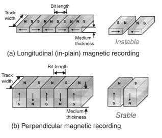
Fig. 5. Longitudinal (in-plane) and perpendicular magnetic recording mode.
