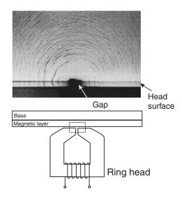
Fig. 1. Fundamental scheme of longitudinal magnetic recording with a ring-shaped head. Magnetic force lines of the ring head in the enlarged model experiment are shown.
