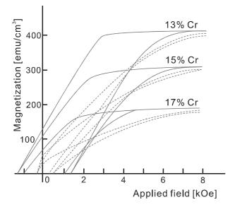
Fig. 8. Perpendicular (solid lines) and in-plane (broken lines) hysteresis curves of Co-Cr perpendicular recording media with various Cr contents.
