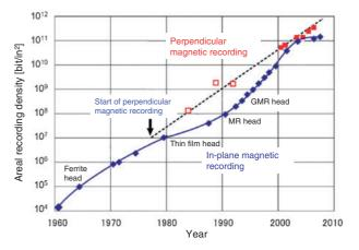
Fig. 22. Yearly growth of areal recording densities of HDD with longitudinal and perpendicular magnetic recording. (□, 50 kBPI × 2.5 kTPI in 1984, 250 kBPI × 7.1 kTPI in 1989, trial product of FDD at Tohoku Univ. and Fujitsu trial HDD product of 2 Gbits/in<sup>2</sup> in 1992; ■, Hitachi and Toshiba—HDD products and prototype; ◆, longitudinal magnetic recording)
