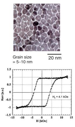
Fig. 20. Plan view of a CoPtCrO/Ru perpendicular magnetic medium using transmission electron microscopy (TEM) (upper) and its Kerr hysteresis curve (lower) by Toshiba.<sup>16</sup>
