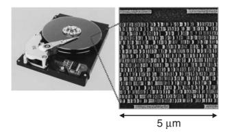
Fig. 19. Prototyping of a hard disk drive using perpendicular magnetic recording  $(52.5 \text{ Gb/in}^2)$  and its recording bit image on the disk, by Hitachi Ltd.<sup>15</sup>
