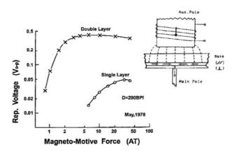
Fig. 13. The first data of recording magneto-motive force versus reproduced output characteristics of a double-layered perpendicular medium and a single-pole head in comparison to a single layer perpendicular medium (May 19, 1978).
