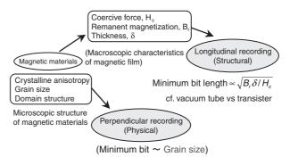
Fig. 16. Conceptual explanation of how the recording upper limit is determined.  $^{\rm (2)}$
