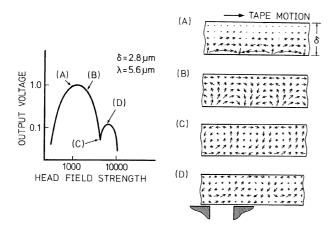
Fig. 3. Recorded magnetization distribution observed using a self-consistent computer simulation ( $\delta$ , magnetic layer thickness in the tape;  $\lambda$ , recording wavelength).
