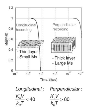
Fig. 18. Stability of perpendicular type recording bits in the phenomena of thermal magnetization decay.  $(M_s, \text{ saturated magnetization; } K_u, \text{ energy of magnetic anisotropy; } V, \text{ volume of particles; } k_B, \text{ Boltzmann constant; and } T, \text{ absolute temperature.})$
