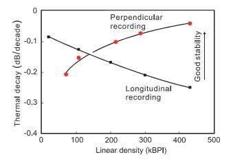
Fig. 21. Thermal stability of recording bits of a hard disk drive, indicating that the higher the density of perpendicular magnet recording, the less the decrease the stability becomes, thereby showing sufficient stability, by Toshiba.<sup>17)</sup>
