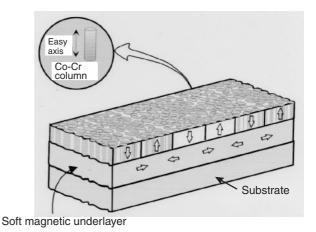
Fig. 9. Double-layered perpendicular magnetic recording medium.
