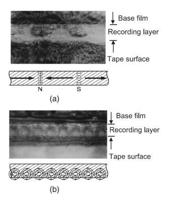
Fig. 2. Bitter pattern images of recorded magnetization at the cross-sectional surface of the magnetic tape: (a) Long wavelength, (b) Short wavelength.
