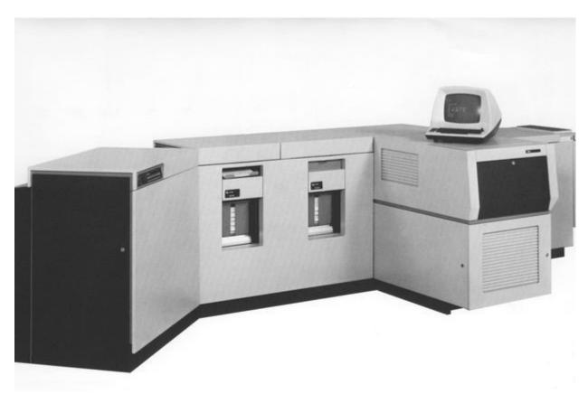
The 9700 laser printer, Xerox's first commercial laser printer, introduced in 1977, weighed more than a ton and was priced at \$295,000. PHOTO: XEROX
