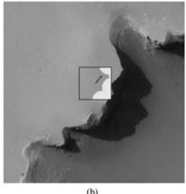
Figure 13. Cost map from the first Field D\* checkout. The Field D\* cost map from the final step is shown in (a). The rover is depicted as a white diamond and the goal as a checkered diamond. The dark areas were imaged and determined to be safe by the rover. The white regions are keep-out zones used to keep the rover away from Victoria Crater. An orbital image captured by the Mars Reconnaissance Orbiter is shown in (b), along with an overlay of the Field D\* cost map. Courtesy NASA/JPL-Caltech.
