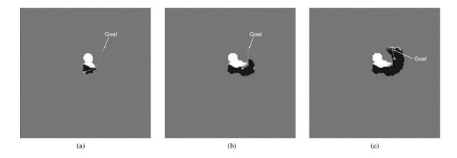
Figure 16. Cost maps from the third Field D\* checkout. The initial and final cost maps are shown in (a) and (c), respectively. A map from the middle of the drive is shown in (b). The checkered line represents the path planned by Field D\*, and the white regions are hazards. The dark areas are safe.
