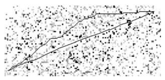
**Figure 4.** Paths produced by classic grid-based planners (uppermost path) and Field  $D^*$  (lower path) in a  $150 \times 60$  uniform resolution grid. Darker cells represent higher cost areas. Figure reproduced from Ferguson and Stentz (2006).
