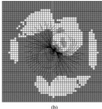
**Figure 10.** Goodness map filtering. Obstacle cells are shown in white. The goodness map in (a) contains regions completely surrounded by obstacle cells. Planning time is greatly increased when arc endpoints fall in these regions. All cells reachable from the rover location are shown in dark gray in (b). Note that the regions surrounded by obstacle are not marked as reachable.
