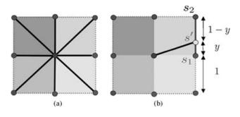
**Figure 3.** (a) The typical transitions (in black) allowed from a node (shown at the center) in a uniform grid. Notice that only headings of 45-deg increments are available. (b) Using linear interpolation, the path cost of any point s' on an edge between two grid nodes  $s_1$  and  $s_2$  can be approximated. This can be used to plan paths through grids that are not restricted to just the 45-deg heading transitions. Figure reproduced from Ferguson and Stentz (2006).
