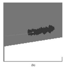
Figure 19. Cost maps from the fourth Field D\* checkout. As the rover approaches the edge of the map (a), it is autonomously recentered on the rover position (b). The planned path is shown as a checkered line (the goal was selected outside the map bounds). The white region is a keep-out zone placed between the rover and Victoria Crater. The dark areas were verified safe by the rover during its traverse.
