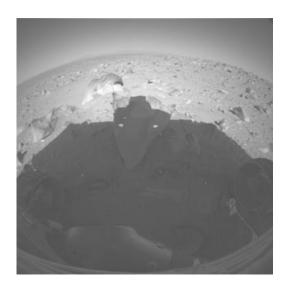
**Figure 2.** On sol 108, Spirit was unable to autonomously navigate to a goal location on the other side of this cluster of rocks. This image was captured by one of the front hazard avoidance cameras mounted on the body of the rover. A portion of the scene is in a shadow cast by the rover. Courtesy NASA/JPL-Caltech.
