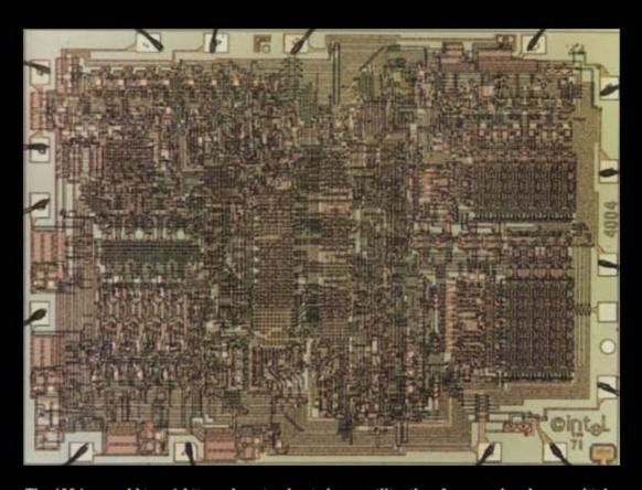
The 4004 can add two 4-bit numbers in about eleven millionths of a second and can multiply only by repeated addition. The chip contains a 4-bit adder (for doing just that), an accumulator (for keeping track of subtotals), and sixteen registers (for temporarily storing results). The two larges registers are the rectangular grids on the far right. The black bars along the edges are wires. Actual size: 0.110 x 0.150 inches.
