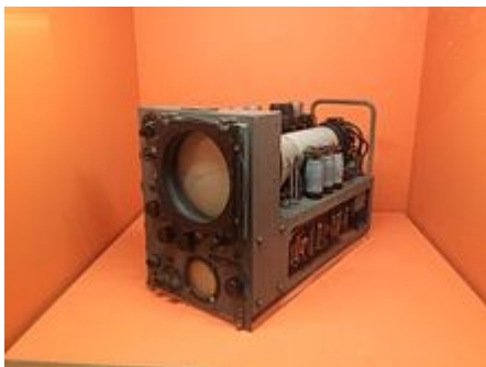
H2S Radar display unit as flown during World War 2, courtesy Wikipedia
