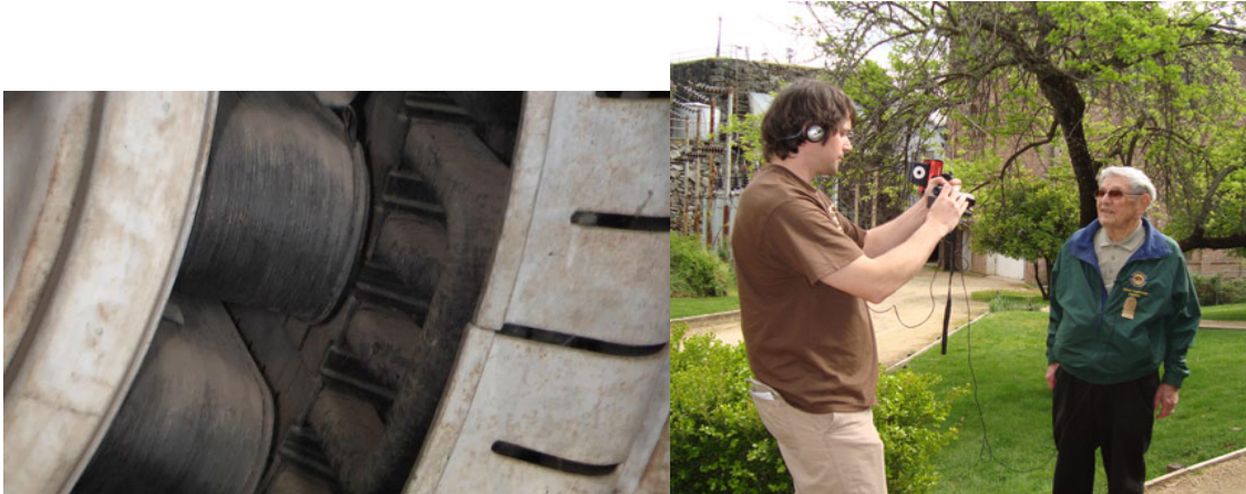
Left: Field Coils on the left, stator on the right. 3 phase Right: Shooting the interview with Bill Henning, PH Docent see the videos at the top of this page .
