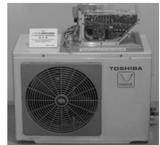
Inverter unit (top) and the outdoor unit mounted with the inverter unit (bottom)
