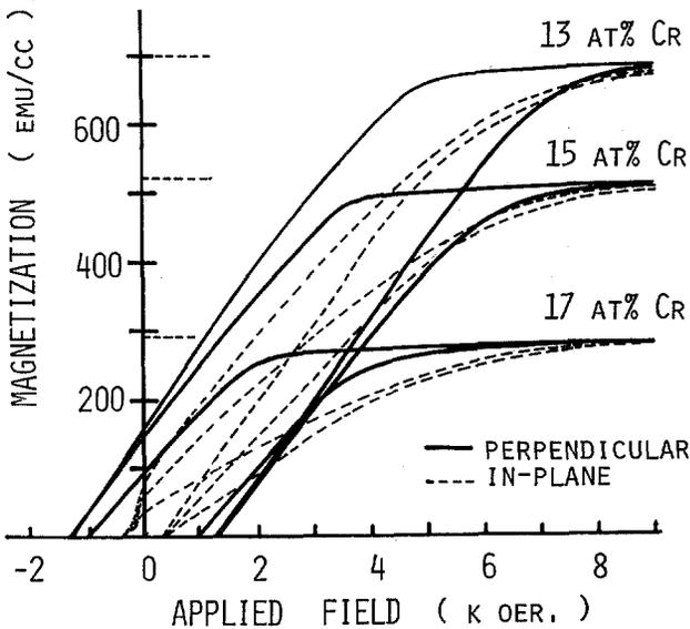
Fig. 5 M-H loops of Co-Cr sputtered films measured by disk samples of 5 mm in diameter (single layer).
