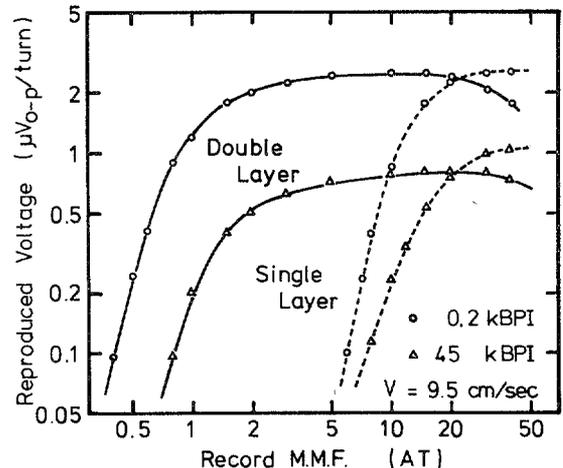
Fig. 9 Reproduced voltage vs. recording magneto-motive force characteristics [Record: perpendicular head, Reproduction: ring head].
