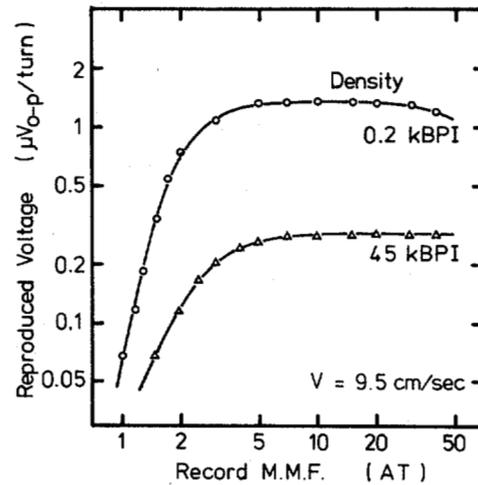
Fig. 12 Reproduced voltage vs. recording magneto-motive characteristics [Record, Reproduction: perpendicular head].
