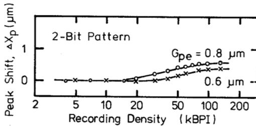
Fig. 11 Peak shift vs. bit density characteristics measured by 2-bits NRZ signal (double layer medium).
