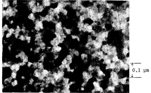
Fig. 6 Transmission image by electron microscopy of Co-Cr film of 0.34  $\mu$ m in thickness.
