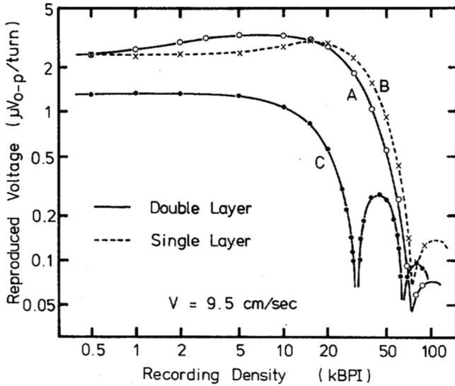
Fig. 10 Reproduced voltage vs. bit density characteristics [Record: perpendicular head, Reproduction: ring head (A, B) perpendicular head (C)].
