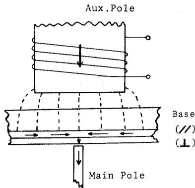
Fig. 7 Flow of flux in double layer medium at recording process.
