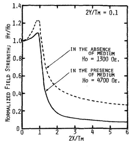
Fig. 4 Effect of the recording medium on the magnetic field distribution around the main pole (model experiment).
