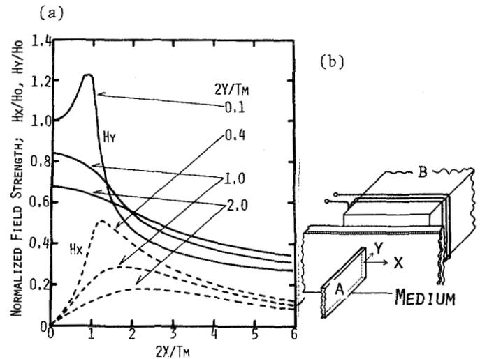
Fig. 3 Magnetic field distributions around the main pole (Thickness:  $T_m$ ) and head construction (over view) (b).
