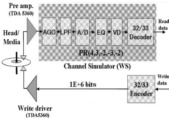
Fig. 4. Diagram of BER estimation system.
