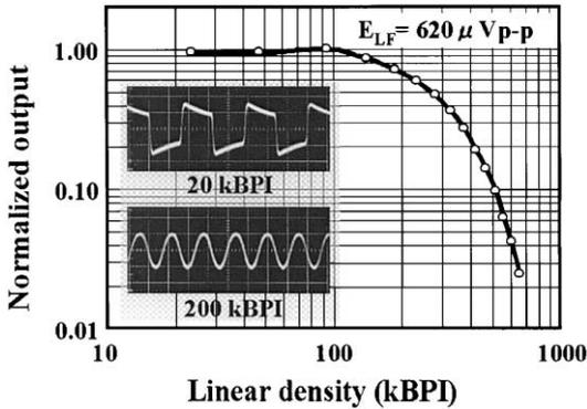
Fig. 3. Roll-off characteristics and waveforms.
