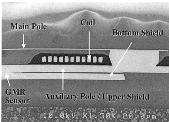
Fig. 1. Cross sectional view of a perpendicular head.
