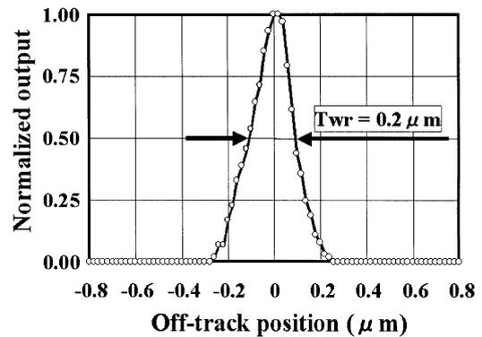
Fig. 6. Micro track profile of GMR head.
