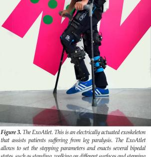
that assists patients suffering from leg paralysis. The ExoAtlet allows to set the stepping parameters and enacts several bipedal states, such as standing, walking on different surfaces and stepping over obstacles. Reproduced with permission from Ekaterina Bereziy, exoatlet.ru.
