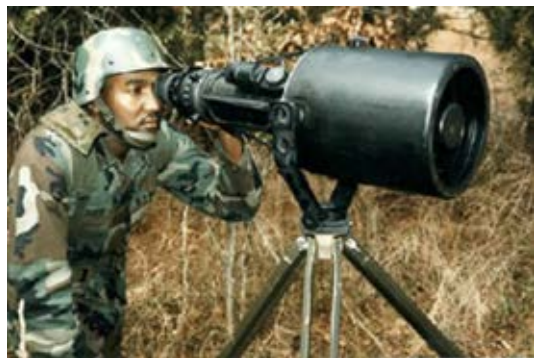
Fig. 13. TVS-4 Night Observation Device – 1 st generation intensifier used only at the night sky illumination. It had an 8" aperture and was 30" long (after Ref. 45).
