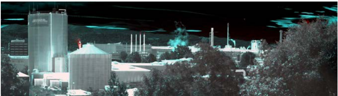
Fig. 36. Bispectral infrared image of an industrial site taken with a 384×288 dual-colour InAs/GaSb SL camera. The two-colour channels 3–4 \mu\text{m} and 4–5 \mu\text{m} are represented by the complimentary colours cyan and red, respectively (after Ref. 109).
