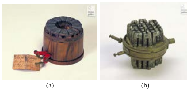
Fig. 2. The Nobili-Melloni thermopiles: (a) thermopile's prototype invented by Nobili (ca. 1829), (b) incomplete version of the Nobili-Melloni thermopile (ca. 1831). Museo Galileo – Institute and Museum of the History of Science, Piazza dei Giudici 1, 50122 Florence, Italy (after Ref. 14).
