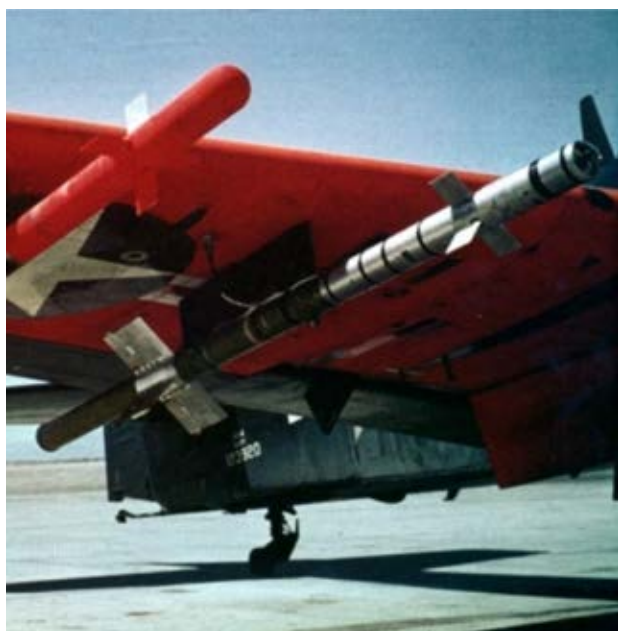
Fig. 14. Prototype Sidewinder-1 missile on an AD-4 Skyraider during flight testing (after Ref. 47).
