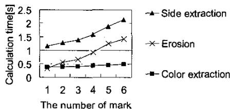
Fig. 6 Relationship between the mark number and the calculation time
