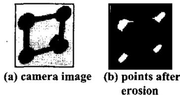
Fig. 4 Mark images using the Erosion method
