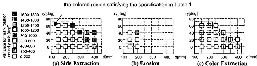
Fig. 2 Experimental results for mark rotation around the y axis
