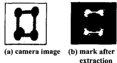
Fig. 5 Mark images using the Erosion method
