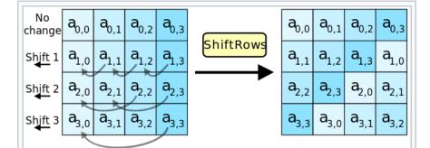
In the ShiftRows step, bytes in each row of the state are shifted cyclically to the left. The number of places each byte is shifted differs incrementally for each row.
