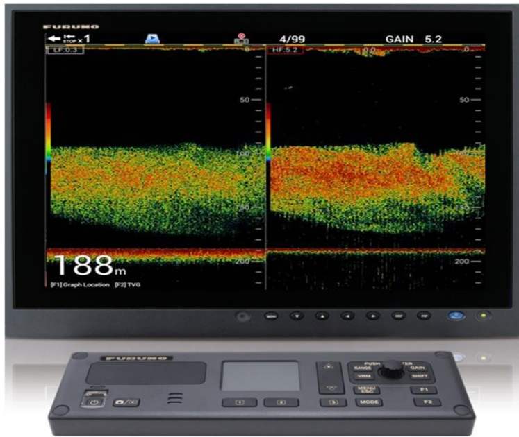
Fig. 5 A picture of fish schools on the fishfinder. (left; 50kHz, right; 200kHz)
