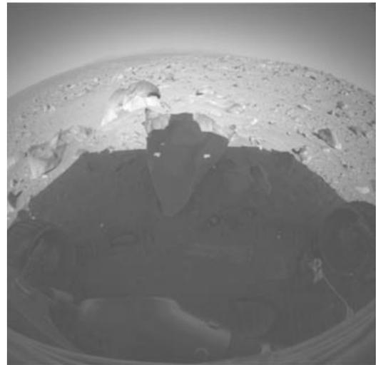
**Figure 2.** On sol 108, Spirit was unable to autonomously navigate to a goal location on the other side of this cluster of rocks. This image was captured by one of the front hazard avoidance cameras mounted on the body of the rover. A portion of the scene is in a shadow cast by the rover. Courtesy NASA/JPL-Caltech.
