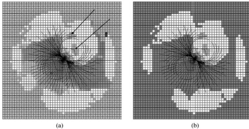
**Figure 10.** Goodness map filtering. Obstacle cells are shown in white. The goodness map in (a) contains regions completely surrounded by obstacle cells. Planning time is greatly increased when arc endpoints fall in these regions. All cells reachable from the rover location are shown in dark gray in (b). Note that the regions surrounded by obstacle are not marked as reachable.
