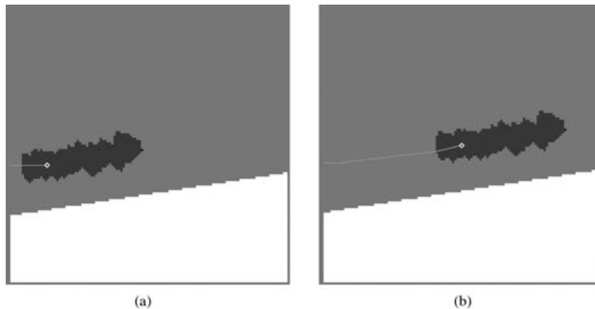
**Figure 19.** Cost maps from the fourth Field D\* checkout. As the rover approaches the edge of the map (a), it is autonomously recentered on the rover position (b). The planned path is shown as a checkered line (the goal was selected outside the map bounds). The white region is a keep-out zone placed between the rover and Victoria Crater. The dark areas were verified safe by the rover during its traverse.
