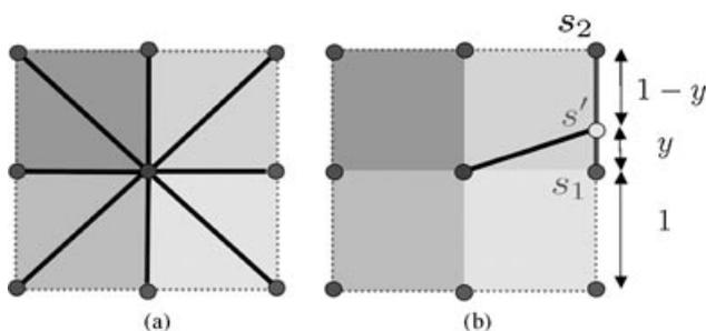
**Figure 3.** (a) The typical transitions (in black) allowed from a node (shown at the center) in a uniform grid. Notice that only headings of 45-deg increments are available. (b) Using linear interpolation, the path cost of any point  $s'$  on an edge between two grid nodes  $s_1$  and  $s_2$  can be approximated. This can be used to plan paths through grids that are not restricted to just the 45-deg heading transitions. Figure reproduced from Ferguson and Stentz (2006).
