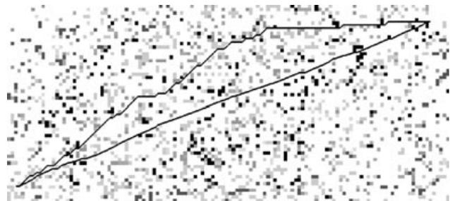
**Figure 4.** Paths produced by classic grid-based planners (uppermost path) and Field D\* (lower path) in a  $150 \times 60$  uniform resolution grid. Darker cells represent higher cost areas. Figure reproduced from Ferguson and Stentz (2006).
