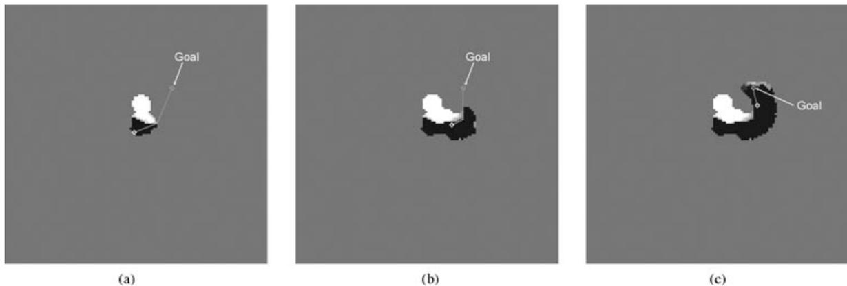
**Figure 16.** Cost maps from the third Field D\* checkout. The initial and final cost maps are shown in (a) and (c), respectively. A map from the middle of the drive is shown in (b). The checkered line represents the path planned by Field D\*, and the white regions are hazards. The dark areas are safe.
