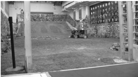
**Figure 11.** MER SSTB rover in an indoor sandbox at JPL.
