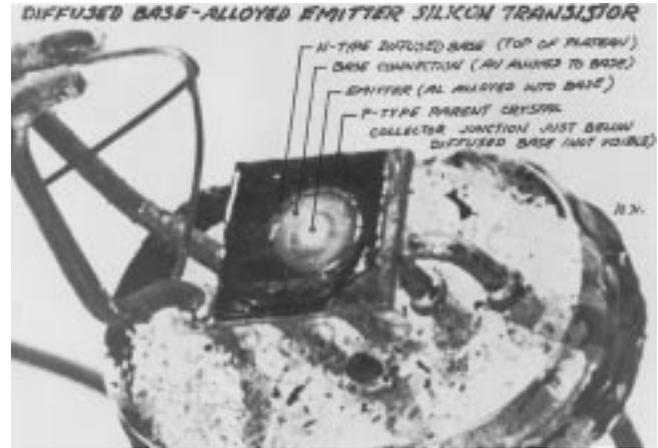
Fig. 3. Diffused-base Si p-n-p transistor with evaporated metal contacts made at BTL in 1955. The hand lettering is simply for the convenience of discussion (cf., Fig. 4). Note that thermo-compression bonding did not yet exist and the leads are spring contacts bent out of place for device viewing.
