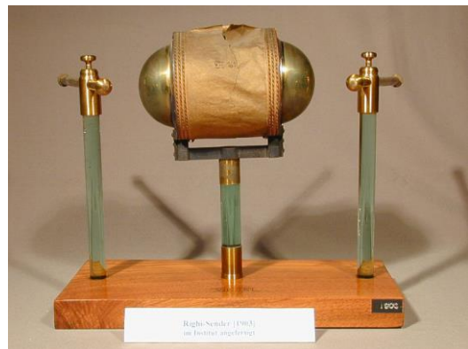
Fig. 3 - Righi's transmitter spark type oscillator made at the institute, 1903, Inv.No: VIII - 161/162
