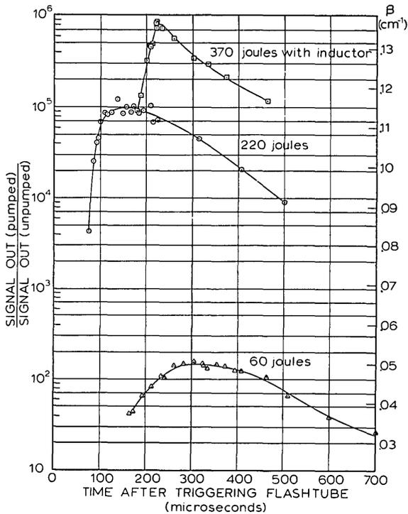
Fig. 9. Gross amplification,  $e^{\beta l_p}$ , in a fiber laser. Length 1 m, core diameter  $10 \mu$ , 2.5%  $\text{Nd}^{3+}$  in a barium crown glass. Bevel angle,  $\theta = 10^\circ$ , on one end. Pump power was supplied by a 7.6-cm straight flashtube (GE FT 91/L). For pumping at 370 J it was necessary to use an inductance in series with the power supply. This accounts for the fact that the peak amplification occurs at a later time than for 220-J pump energy.
