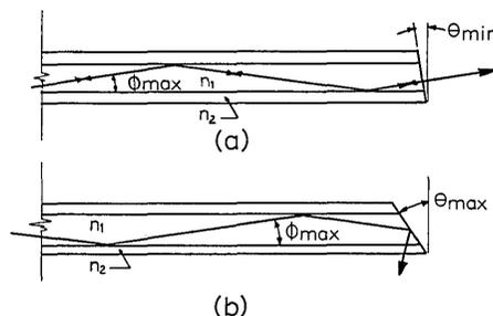
Fig. 8. Limits on bevel angle. In (a) the extreme meridional ray is reflected back on itself. All other meridional rays are, therefore, reflected at angles such that they do not undergo total internal reflection at the core-cladding interface. In (b) the extreme meridional ray is totally internally reflected at the end surface. If the angle  $\theta$  is made larger than this value, more of the useful rays will be totally reflected and thereby lost for purposes of amplification.
