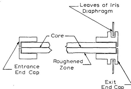
Fig. 3. Arrangement of end caps on fiber lasers. The iris diaphragm is mounted on the front of the photomultiplier housing, and together with the exit end cap it provides a light trap.
