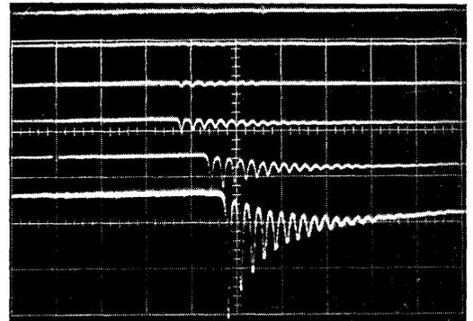
Fig. 5. Amplification at several pumping levels. Each trace represents the signal out of the fiber laser amplifier. Starting from the top, the pumping levels were 0, 5 J, 10 J, 15 J, 20 J, and 25 J. The input signal and oscilloscope sensitivity were the same in each case. For fiber data, see Fig. 6.
