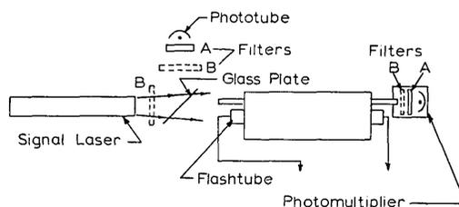
Fig. 2. Experimental setup for measuring amplification. Signal laser: 6.35-mm diam core, 9.5-mm diam cladding, 30.5-cm long. Filters, A, in front of the phototube pass only the 1.06- $\mu$  laser radiation. Filters, B, partially absorb at 1.06 to keep the signal within the linear range.
