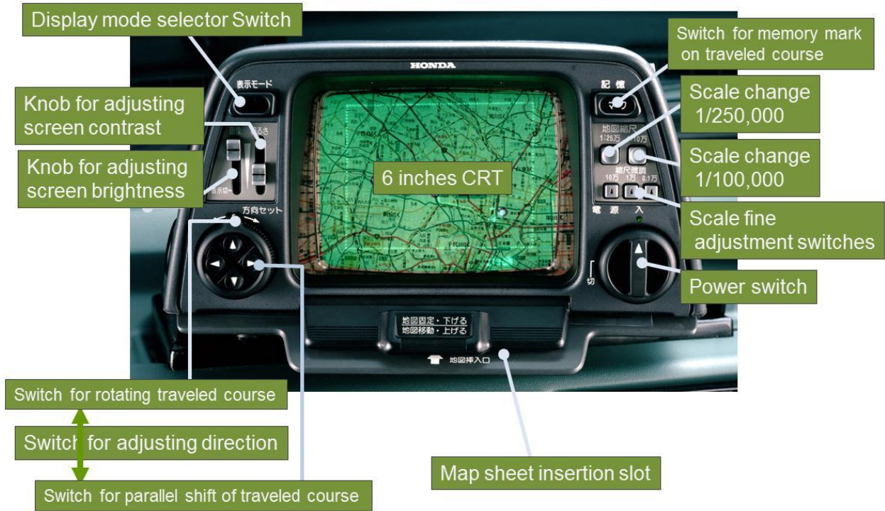
Fig. 9: Switches configuration of display equipment (front view)
