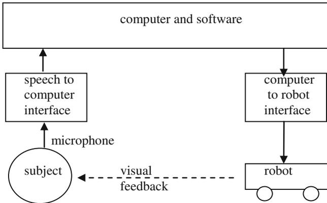
Fig. 2. A system diagram of the 1986 speech-to-robot interface
