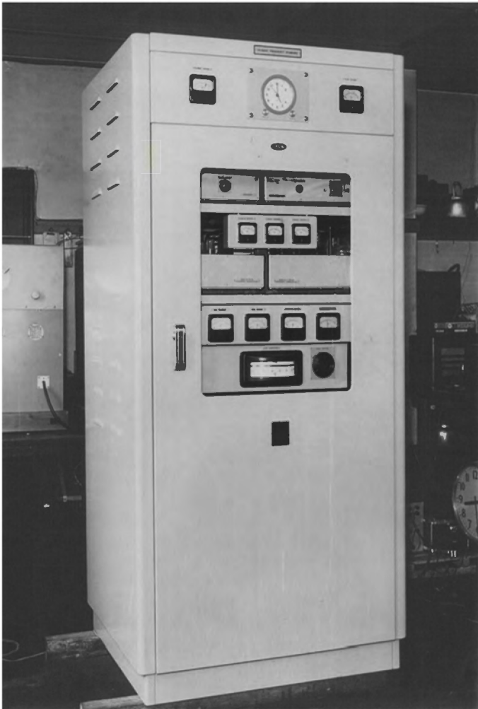
Fig. 7 Koga's final model KQ-6 installed at KDD Co. Ltd., providing time and frequency standards
