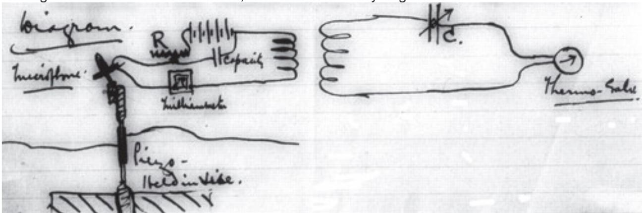
Figure 2. Boyle's drawing of his measurement with the piezo-electrique (on the lower left side), which is connected to a microphone. The microphone, which forms part of an RCL circuit on the left, generates alternating current in the circuit as a result of its mechanical movement. Through the coils this current induces an electric current in the CL circuit to the right; a thermoelectric galvanometer is used to measure the current. (From Boyle to Rutherford, 12 December 1916.)
