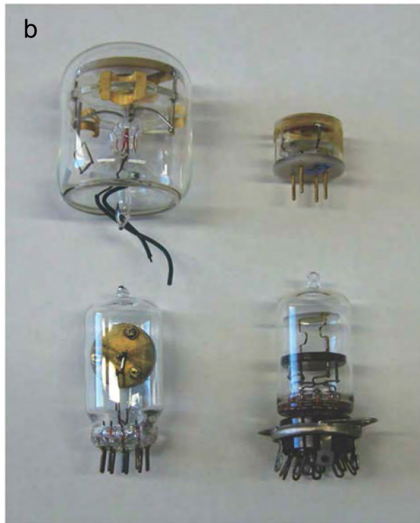
Enclosed-type tubes made at Koga's Lab
